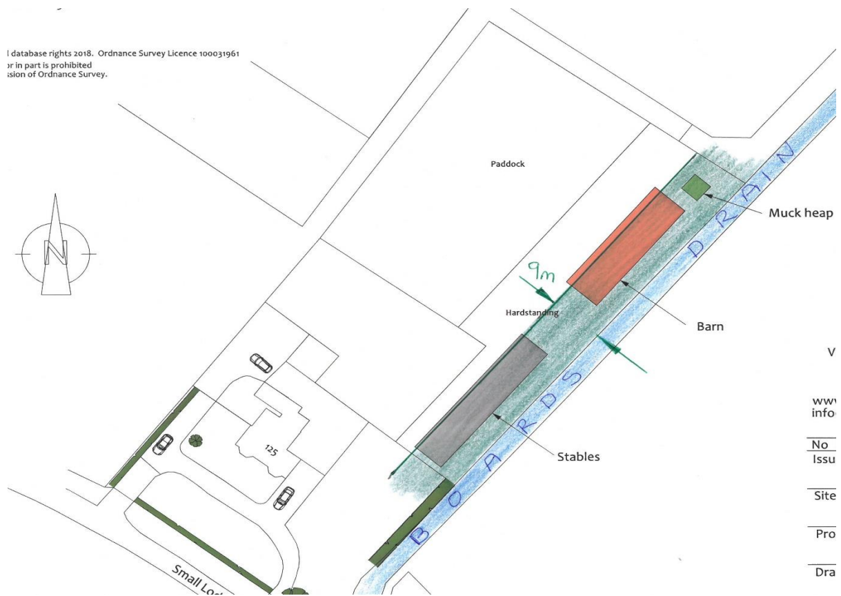
An amended extract from Anglia Building Consultants' Drawing No. 19-1879-2 showing the location of the Board's Drain and potential encroachment within the Board's maintenance access strip.
