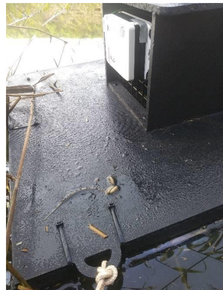
Figure 1 & 2: New mink raft in operation. Note otter guards in place. Remoti unit attached to rear (2).
