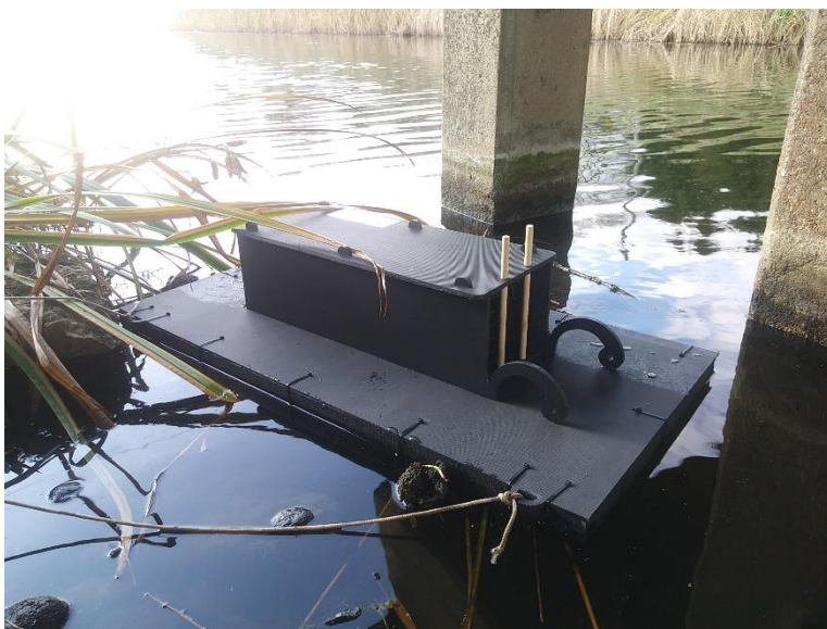
Figure 1 & 2: New mink raft in operation. Note otter guards in place. Remoti unit attached to rear (2).
