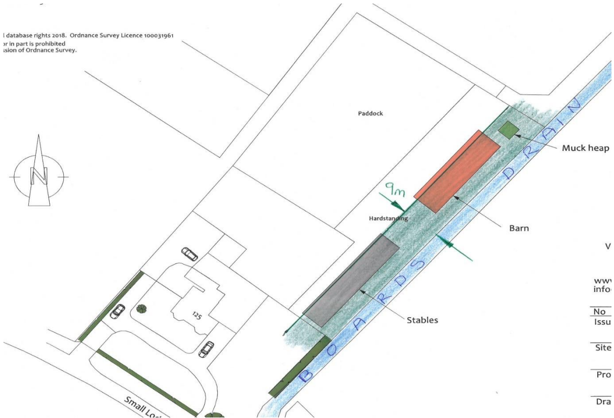
An amended extract from Anglia Building Consultants' Drawing No. 19-1879-2 showing the location of the Board's Drain and potential encroachment within the Board's maintenance access strip.
