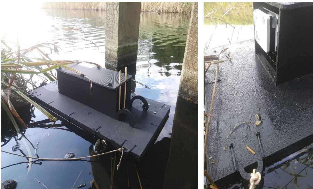
Figure 1 & 2: New mink raft in operation. Note otter guards in place. Remoti unit attached to rear (2).
