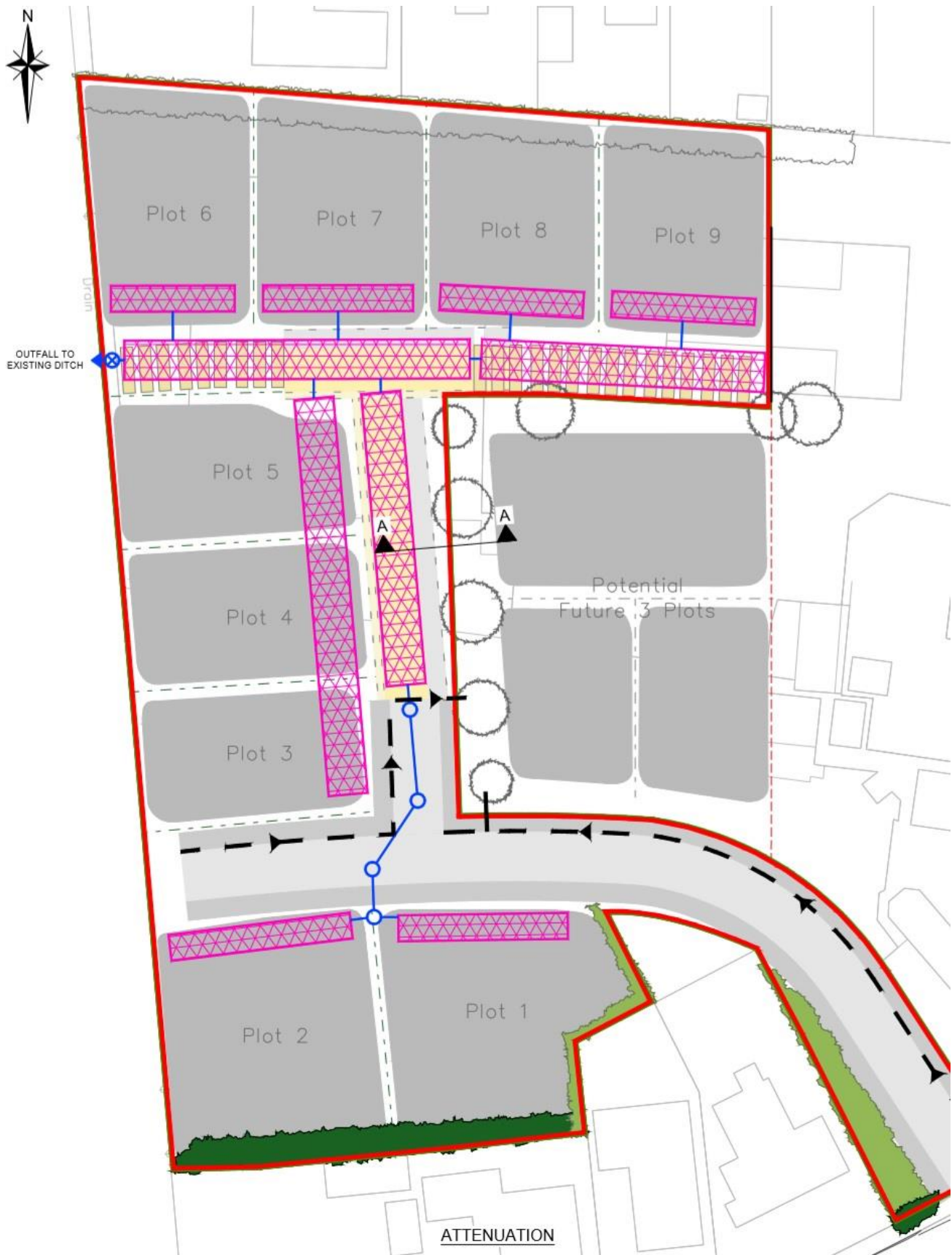
Extract from Cannon Consulting Engineer's Drawing Number V551 - PL - SK - 300 Rev. P01 showing a suggested SuDS layout
