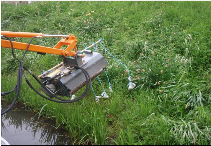
A flushing pass with suspended golf balls and bells checks for nesting birds before mowing takes place.
